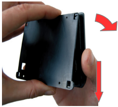
C) Slide the display frame downwards with respect to the cover and release it.
