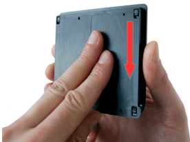
A) Slide the display frame upwards with respect to the back cover
