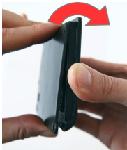
B) Lift the lower part of the display frame
